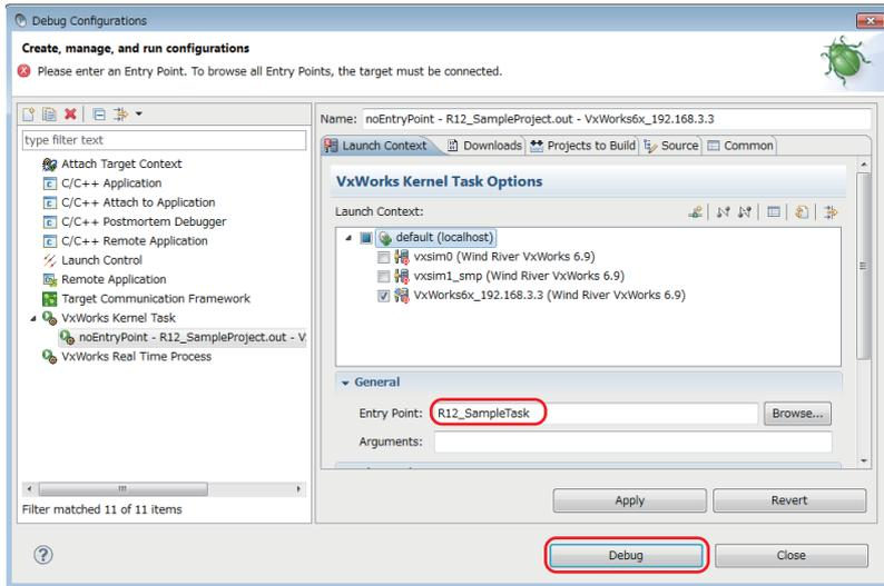
8. Debugging starts. Program execution stops at the start of the function specified for "Entry Point".
