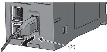
1. Check that no USB Mass Storage Class-compliant device is accessed.
