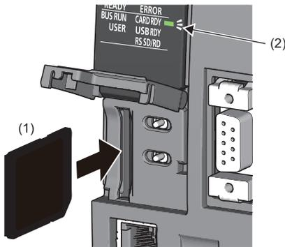
1. Insert an SD memory card (1) straight into the SD memory card slot with its cutout pointed down. Make sure it is not uplifted after inserting it.
