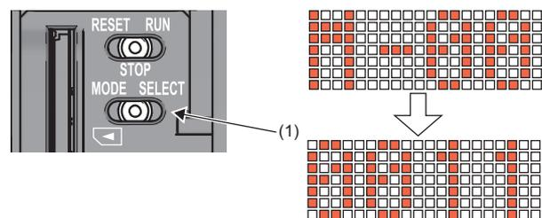
5. Set the RESET/STOP/RUN switch (3) to the RUN position. The selected mode is executed. The BUS RUN LED (2) will be flashing during initialization.
