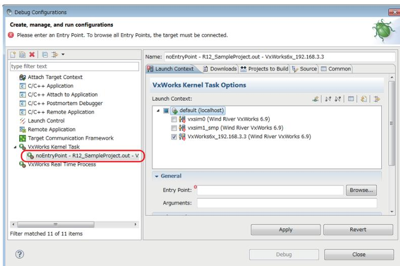
4. Select a target server indicating connection to the C Controller module.
