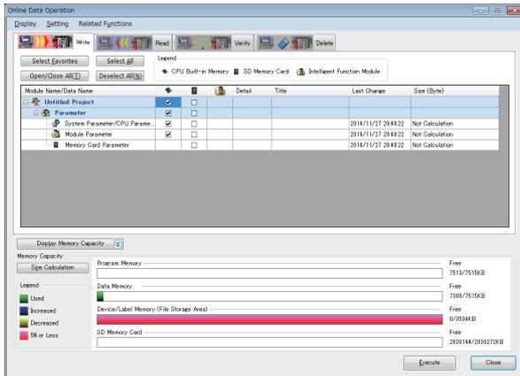
1. Select "System Parameter/CPU Parameter" and "Module Parameter".
