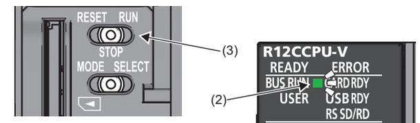
6. Check that the BUS RUN LED (2) turns ON and "0000" is displayed on the dot matrix LED, then reset the C Controller module. (Page 41 RESET/STOP/RUN switch)
