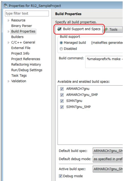
4. Select only the checkbox of "ARMARCH7gnu\_SMP" in "Available and enabled build specs".
