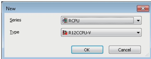
1. Select the C Controller module to be used in the "New" screen, and click the [OK] button.
