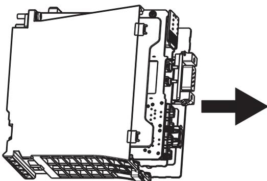
2. Remove the printed circuit board from the case.
