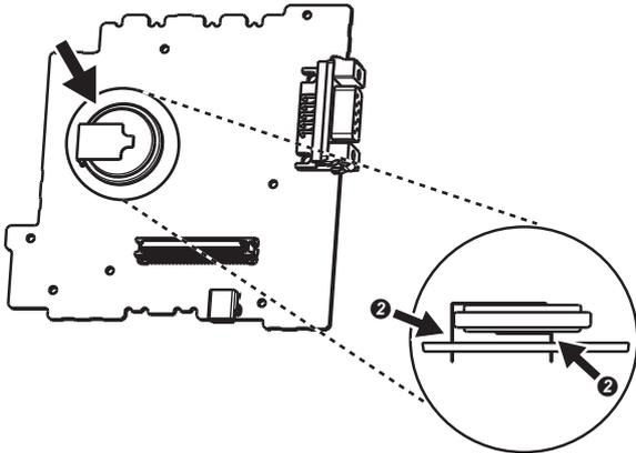
5. Cut off the ② (lead) portion of the battery, which is attached on the surface of the printed circuit board with RS-232 connector, using a tool such as nippers, and remove the battery.
