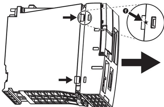
1. Lift the ❶ (★) portion on the side of the C Controller module, and remove the front cover.
