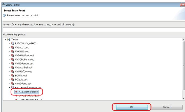
7. Check that the function name selected in step 6 is set for "Entry Point", and click the [Debug] button.
