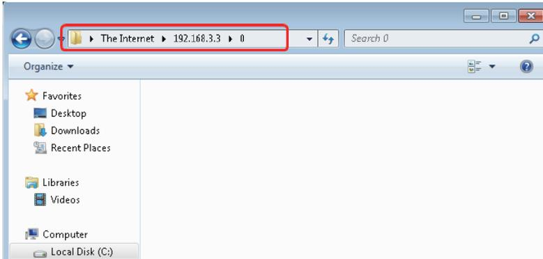
2. Copy the created user program "R12\_SampleProject.out" to the program memory '0' in the C Controller module by a drag and drop operation.
