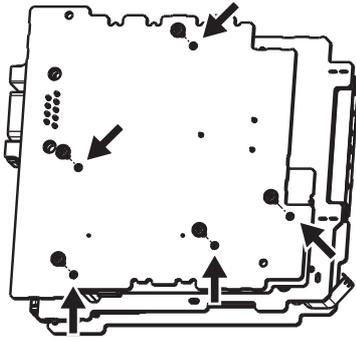
3. Remove five board fixing screws (M2) from the board.
