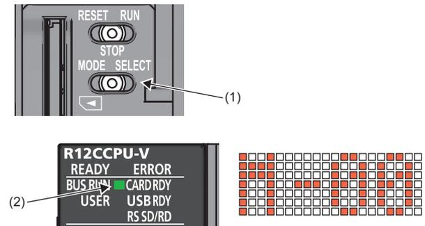
**Point** When the power of the C Controller module is ON, the ERROR LED may flash and an error code may be displayed on the dot matrix LED. (Page 33 Abnormal completion of initialization process)
