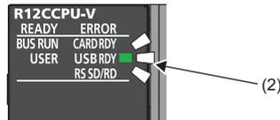
1. Connect a connector of USB Mass Storage Class-compliant device or USB cable to the USB connector (1). Firmly insert the connector to prevent it from falling out.
