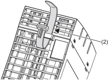
3. Pass the USB cable (3) through the fixing band to fix.
