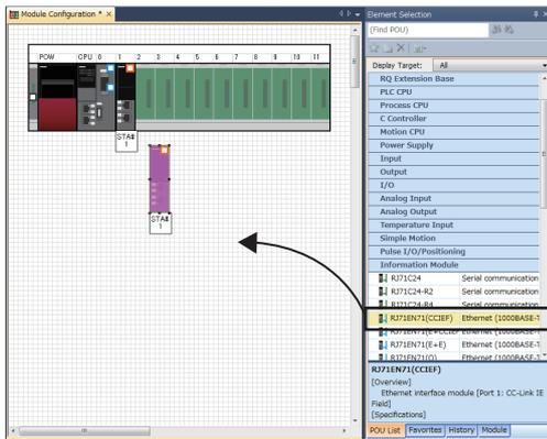
1. Select a base unit to be used from the Element Selection window, and drag and drop it onto the Module Configuration Diagram.
