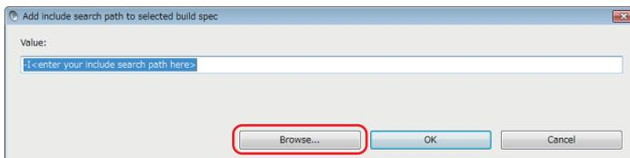
3. Select the include folder for the C Controller module in the "Select directory" screen, and click the [OK] button. In this procedure, the include file is stored in "C:\MELSEC\R12CCPU-V".
